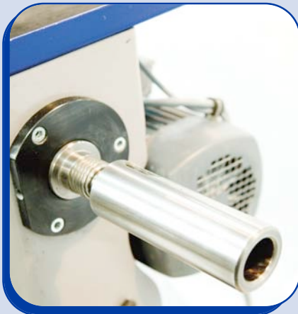
Practical quick locking mechanism for Morse Taper 3 (not included)
