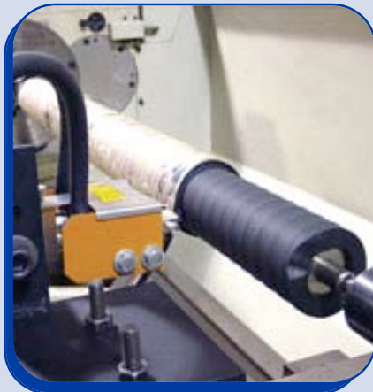
Roughing of 30 shore rubber on offset roller
